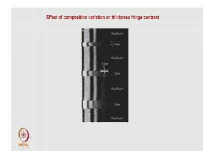
That is what you can see it here, you see this. This gallium arsenate, this is aluminum gallium arsenate. Now you can see that how the fringes are changing. So, gallium arsenate has got a higher this one so fringes spacing. So, here you see that when the aluminum is introduced the fringe spacing has changed, correct?
