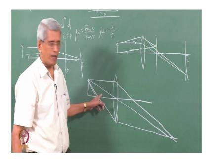
They will all be brought to a focus at a particular that is this ray. So, all of them will be coming this is what how we define as an image plane. So, this is how draw the ray because the first we know the object at what position it is kept and with respect to the lens then we can find out where the image plane is going to be there.
