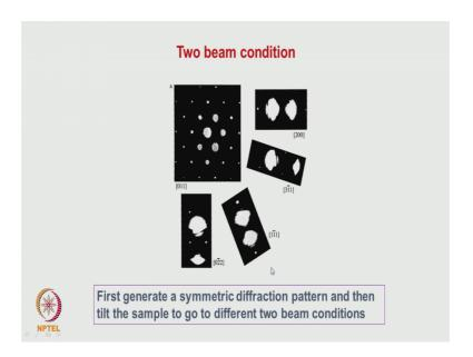
So, I mentioned about the first step is to get a symmetric diffraction pattern, this symmetric diffraction pattern we can get it in a microscope by tilting that sample observing it on that screen and. So, that we get spots which are of uniform intensity how to get this pattern using kukuchi pattern all these things are being covered in a different class we assume that we have for this lecture we assume that we have got a symmetric diffraction pattern ok.
