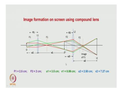
So, how to draw the ray diagram? With this way we can draw the ray diagram and what is image plane image plane is one which all the rays which are emitted from the sample in different directions.
