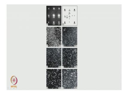
So, what I am showing it here is just an example of a diffraction pattern which has been taken. Why I am showing this picture is essentially to know that in this you forget about these pictures you just concentrate on this diffraction pattern, this diffraction pattern contains lot of spots some spots are very strong some spots are weak. What I have done it is go on to two beam condition put an aperture around the central spot and imaged it that is where I get this bright field picture.
