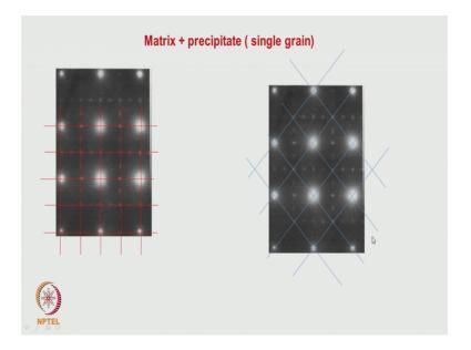
The first thing which I can do it is that, here again the same pattern I take it I can put make a this is a periodic fact pattern. So, I am just showing a grid to identify them if you this is the matrix one here there are some spots which come in between like this, this is one type of a pattern which I can identify at this corresponds gamma prime also which we had seen just now that type of pattern could be seen.
