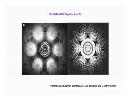
And many patterns if we have to analyze it completely we have to do a compute the simulation also. This simulation has been done I think taking some 30 directions for the beam for the convergence angle. Then you can see that there is a good one-to-one matching between the experimentally observed and the theoretically determined convergent beam pattern.
