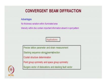
This we call this we will come back later I just mention what all applications applications are precise lattice parameter determination, crystal structure determination thickness of the file could be measured accurately point and space group could be determined. I will just give just a brief idea about some of these aspects especially the point groups
