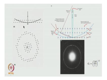
suppose I make the camera length very small that is distance from sample to the screen very small, then what is going to happen is that in the same area instead of only the central spots which are enlarged now because you can see that some of this spots are also being cut by the Ewald's sphere they will also appear. So, this is the 0 th.
