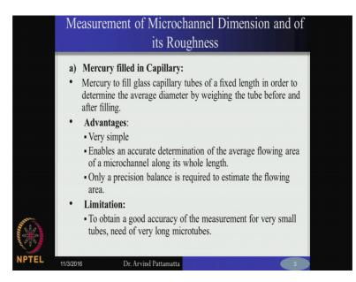
Therefore, very important first step process in measurement is the measurement of the micro channel dimension and its roughness. If you are given a micro channel from the manufacturing section, what you have to do is first may ensure that if you are asked for 100 micron channel you get it, 100 micron plus off course there is always tolerance manufacturing tolerance which has to be accounted.
