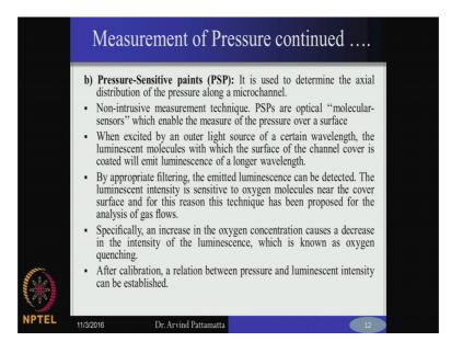
In such a case, you have to use other techniques. The other technique 1 such technique is call the pressure sensitive paint. This is not so commonly used you know in our institute for example, but and this also requires highly sophisticated equipment compared to simple differential pressure transmitter in the earlier case.
