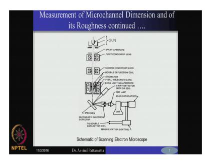
Just to show a schematic of how the scanning electron microscope looks. This is there is a separate theory for this and again the setup is not fairly that large, but also it is ya, it is reasonably its reasonably large, you need to have dedicated, I mean facility for that, room for that and you know you have to maintain the ambient conditions you know at constant temperature and humidity. Yeah you have to invest certain amount of money in maintaining this kind of microscopes.
