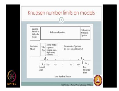
And again this is another float which shows you the instead of the length scale now we used a different parameter which we are now introducing this is called the Knudsen number. So, Knudsen number is a non dimensional parameter. So, which is defined the as the ratio of your mean free paths to the characteristic length scales that you are using.
