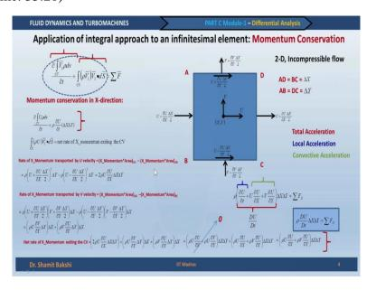
So the first component is the local acceleration which considers the rate of change of velocity within the control volume with time and the  $2^{nd}$  part constitute of the convective component
