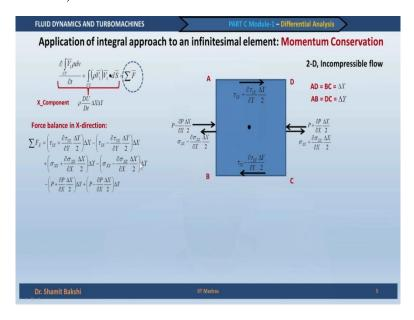
So this is our complete expression, we have got the, for the X component we have got an expression for the left-hand side which is basically mass into the total acceleration. We have to find the forces now. So we do a force balance in the X direction because we are
