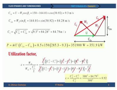
Continuing further we can say that C1U is U, C1U is this portion, C1U is nothing but U - W1 cos beta 1 and we get C1U to be 9.3 metres per second. C1 M is W1 sin beta 1 and we get 84.28 metres per second. And we see that C1U, C1 is equal to 84.79 metre per second. We get power equal to M dot U times C2U - C1U which gives me 351.9 kilowatts.
