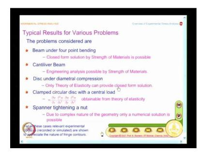
We have discussed in the last class, the problems considered are Beam under four-point bending, Cantiliver Beam, Disc under diametral compression. (Refer Slide Time: 00:36)
