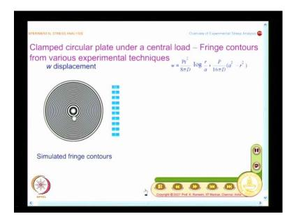
And when I go and find out I get this pattern like this. So what I have here is, I said nature is so good that it gives you. So I have simulated fringe contours, I have concentric circles nature is so good. In the case of beam under bending, you saw horizontal lines. In the case of clamped circular plate, you see beautiful circles. This is again a function of load apply, so you have concentric circles that they come and this is what you have. As a load is increase you have more and more circles.
