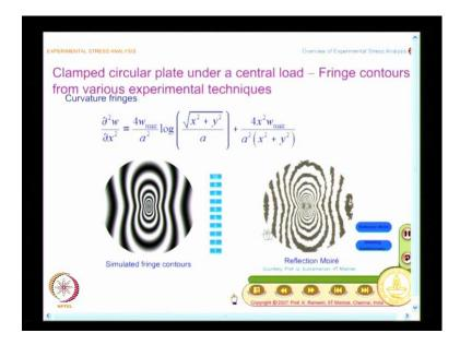
And the simulated fringe contours are like this. If you go to experimental technique you have a nice sort of curvature fringes up time.
