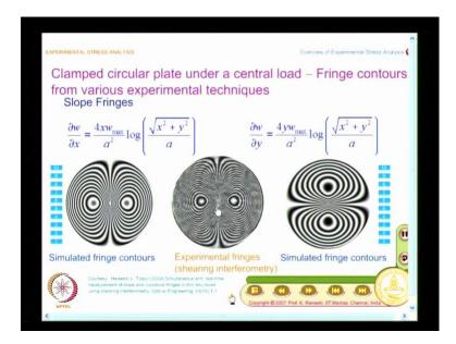
And what you find here is, a very recent experiment on speckle interferometry as given very nice set of contours on thin wafers. And you know in fact it matches very well with what you have as the simulated patterns. This is how you see in the experiment, and this is from the work of Hareesh V. Tippur, he is a best friend of mine.
