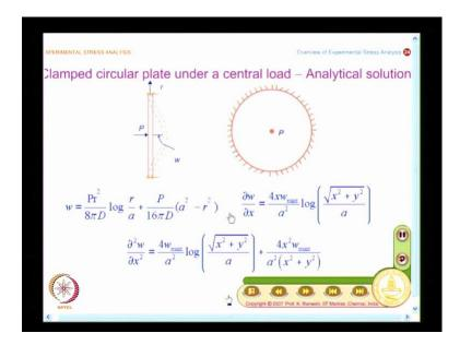
And the next problem what we would take on is, we would take on the problem of a Clamped circular plate under a central load. And what I would appreciate is I have this clamped circular plate, this is clamped at all around the periphery and it subject to a central load. In fact, in the kind of problems where they do out of plane displacement they take this as the bench mark example and using this only they testify their methods.
