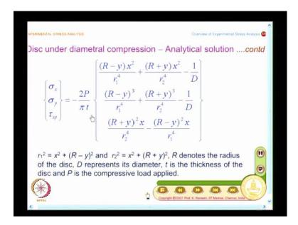
Fortunately, theory of elasticity provides the solution and here again it is given in a convenient form sigma x, sigma y tau x y and you have this as minus 2 P by phi t and I would request all of you to take down this equations. Though these equations are very long, very valuable information when we develop photo elasticity we could directly use these equations for our interpretation.
