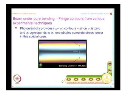
We now go back and see what photoelasticity gives; it gives you contours of sigma 1 minus sigma 2. In the bottom half of the beam you have sigma 1 corresponds to sigma x and sigma 2 is 0 and sigma 1 and sigma 2 contours appear horizontal and you see some deviation from straight line in this zone.
