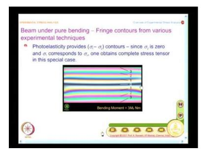
Because, this is closer to the load application point in the experiment and what you see here is, I have increase the load in steps of 1 and you find that this is fringe order 0, fringe order 1, fringe order 1 at the bottom and when I double the load, I see the fringes doubled. So, it is a function of load and I can also label them and when I triple the load the fringes are increasing from 0 to 3 on either side.
