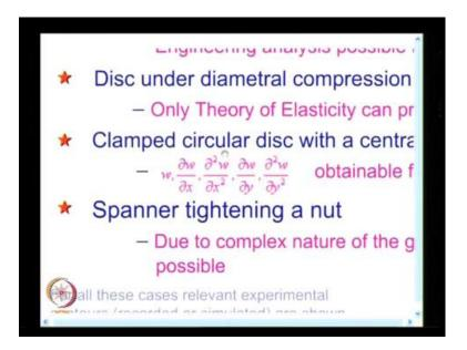
I can find out w that is out of plane displacement, dou w by dou x is slope, dou square w dou x square is curvature, similarly I have curvature in the other direction dou w by dou
