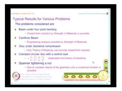
I can go and I have taken in all five problems, and they are also done with graded level of complexity. So, one of the simplest problem which I have taken is a Beam under four point bending. That is a first problem to start with and why I have taken this is you have close from solution by strength of materials. So, that is what you have done in a course in strength of materials.
