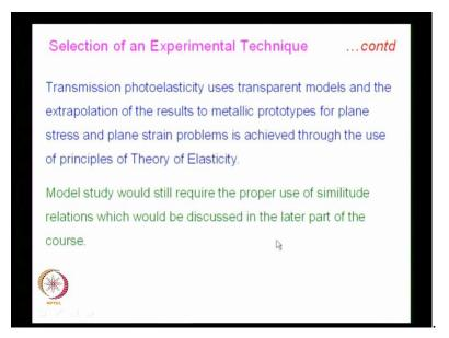
Transmission photoelasticity uses transparent models and the extrapolation of the results to metallic prototypes for plane stress and plane strain problems is achieved through the use of principles of Theory of Elasticity. You are actually using a model, and model study would still require the proper use of similitude relations which would be discussed in the later part of the course.
