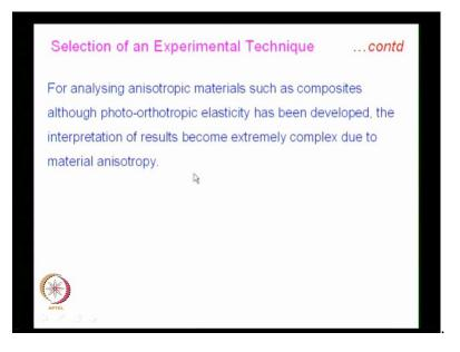
For analysing anisotropic materials such as composites although photo-orthotropic elasticity has been developed. The interpretation of results become extremely complex due to material anisotropy.
