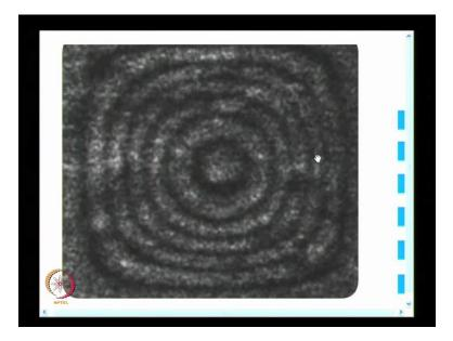
And what you have here is, in all these modern techniques they employee computers. Because of computer processing the double exposure technique is done digitally. So, initially is stored the initial configuration in a file, and use it for viewing the deformed configuration. It is easy to see fringes in real time as the model is loaded.
