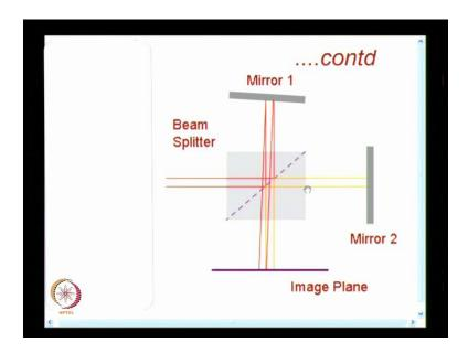
So, you have the ray goes and hits this mirror, this is kept perpendicular and the mirror one is slightly tilted. So, beam splitter sends one ray to this mirror, and sends other component to this, and whatever comes from this because of the tilt, it gets shifted and this is called; it is also said it is shear to this point. So, for each incident ray you will have two rays impinging on the image plane.
