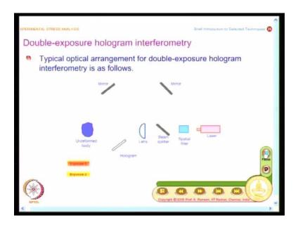
By using a suitable optical arrangement we can get the some of principles stresses that is; sigma 1 plus sigma 2, which are known as Isopachics. If we use this technique in conjunction with photoelasticity, then we can get the individual principle stresses.
