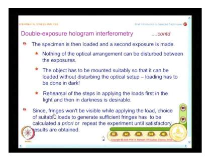
The other difficult point here is, since you do not know a priori how the fringes are formed. You will have to have appropriate calculation to find out, what is the extent of load that you should apply and what is advised is, you have to do rehearsal of the steps in applying the loads first in the light and then in darkness is desirable, so you have to do some practice.
