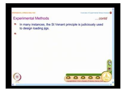
In many instances in designing loading jigs, you use St Venant principle. What it says is? At distances away from the point of loading the distribution is similar to what we finally want. So you will have to use St Venant principle and design your loading jig appropriately so that it simulates service load condition as closely as possible.
