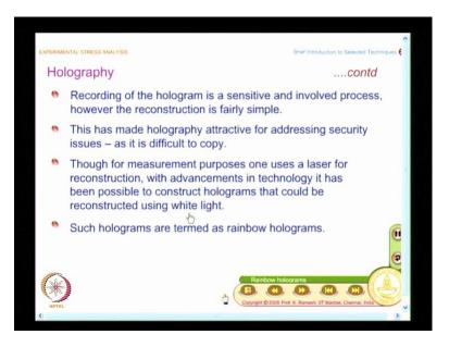
Now, what we want to see is recording the hologram is a sensitive and involved process it is not a that is why it is used for security devices; however, the reconstruction is fairly simple thought for reconstruction I need an optical arrangement to do it.
