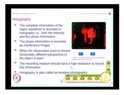
So, what I find is the recording medium should have a high resolution to record this information, because I am recording both the information of intensity and phase. So, I need to have a high resolution to record the information. Holography is also called as
