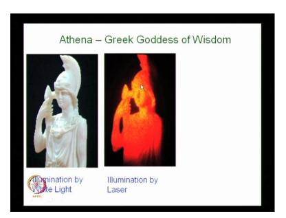
This figure is much better, this figure is not even nice to watch and what you find here is you can see very clearly, there are specular information that is; you see dots, red dots laying on that. And this is what happens, with any laser illumination when you illuminate anything with laser. Laser is highly monochromatic and highly coherent, but you have this information available only in this fashion, and this is your positive.
