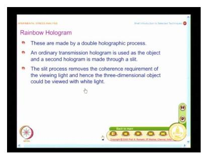
So, what you have here is the slit process removes the coherence requirement of the viewing light and hence the three dimensional object could be viewed with white light. So, that is the advantage.
