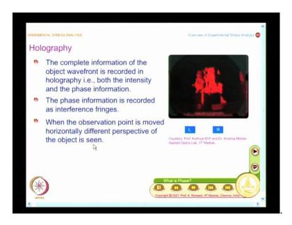
I have a Hologram here, and what is important point here is, first observation is the image is not good; as good as what I record in normal white light. But because I record the phase information, when the observation point is moved horizontally different perspective of the object is seen. So, you are able to get the three dimensional effect of
