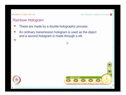
What you have here is these are made by double holographic process, an ordinary transmission hologram is used as the object and a second hologram is made through a slit; it is an optical requirement. And the focus here is I want to see the reconstruction without going into complicated optics just normal white light should be good enough, that is the purpose behind it.
