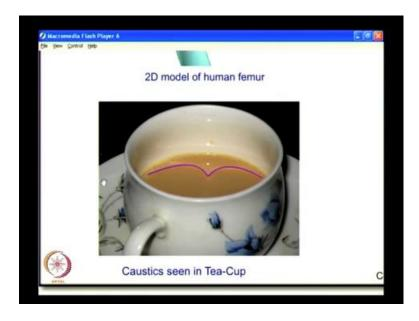
So, what is done is any physical information which could be exploited for measurement is identified and that is translated into an experimental technique. What you see here is a cusp in a Tea-Cup and this you see as a silver line, what happens is when light gets reflected on the curved surface, it gets reinforced and you have a cusp. This can be seen on any shallow filled containers with appropriate lighting and this phenomenon is called Caustics.
