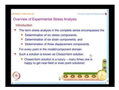
So, the term stress analysis in the complete sense encompasses the determination of six stress components. Why they are six? Why do I say that you have six stress components? Suppose, I take a member like this and then apply a tension, you all know the stresses are developed and what is the value of stress? Someone can answer. Suppose, I apply the load as P and area of cross section is A. What is the value of stress?
