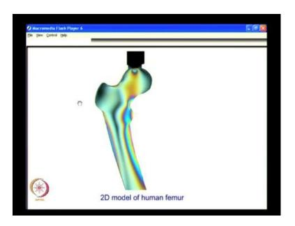
What we see here is stress patterns observed in a 2D model of a human femur. So, you get stress information in stress analysis, and you also get displacement information in stress analysis and what you find here is, for a circular plate clamped at the boundary with a central load. You get the displacements and you can also have the slope. You can also get curvature.
