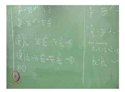
So, my equations are P 1 by rho 1 equals gamma plus 1 by 2 gamma a star square minus gamma minus 1 by 2 V 1 square by 2 and P 2 by rho 2 into gamma plus 1 by 2 gamma into a 1 star minus gamma minus 1 by 2 V 2 V 2 by V 2 square by 2. Now, I am going to multiply this equation with divide by V 1 n and the second equation by V 2 n. So, that I would get P 1 divided by 1 by V n a star square by 1 V 1 n minus gamma minus 1 by 2 V 1 square by V 1 n.
