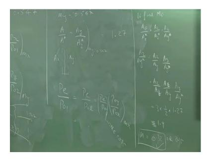
Now, there is something to find M exit I need to find A exit by A exit star which is nothing but, what is we called it as A 2 by A 2 star, A 2 star is also is my A y star. So, I need to find A 2 by A y star which I can rewrite it as A 2 by A y into A y by A y star, I can write it as a by A 1 into A 1 by A y into A y by A y star. So, I need to find A exit by A exit star, so I replace this A quantity in terms of quantities I know.
