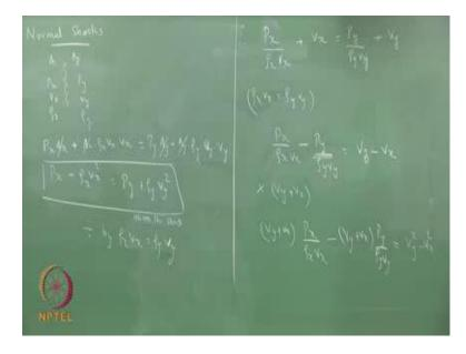
So, like before, I start with the shock here, which has a control volume that is very close by. So, my A x is same as my A y; and, I have a P x here, P y here; v x and v y; rho x and rho y. I apply the momentum equation. I would get P x A x, plus A x rho x v x into v x, which is equal to my P y A y plus A y rho y and v y, multiplied by v y.
