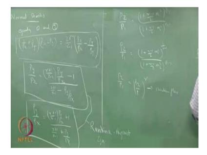
So, equating equation 1 and 2, which I have just now written, this would be 1 by rho x, plus 1 by rho y, into P x minus P y, is minus of the other one. So, it would be 2 gamma by gamma minus 1, into P x minus P x by rho x, minus P y by rho y. So, I have included the minus sign inside the bracket.
