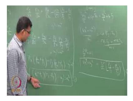
So, this would be v y by v x into P x by rho x, plus v y v x, v x v x cancels. So, it would be P x by rho x minus v x into v x by v y into P y by rho y minus P y rho y equals v y square minus v x square. Now, from the continuity equation, which I have written here, my v x by v y is also my rho y by rho x. So, wherever I see this ratio, I substitute that in terms of rho y and rho x.
