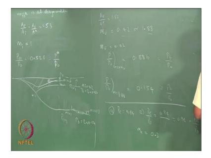
So, the M exit will have 2 values, M exit will have 2 values subsonic value and supersonic value. So, A E by A star 1.53, 1.53 gamma equals 1.4, 1.53 is m equals 0.42 or 1.53. So, I look at this table m equals 1.53, m equals 1.88 which means this is m equals 0.42, this is a isentropic solutions, this is my 1.88. So, this area ratio decides these 2 mach numbers. So, that is decided by this.
