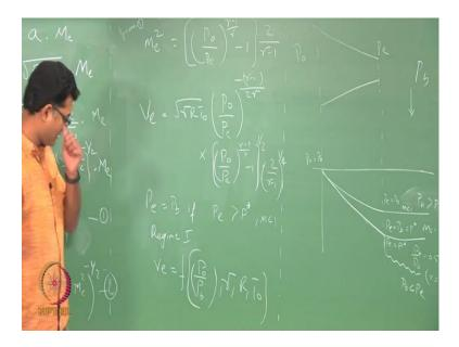
I will also get M e square from this equation. So, from 1, 2, so M e from equation 1, M e square is P 0 by P to the power gamma minus 1 by gamma minus 1 multiplied by 2 by gamma minus 1. So, I substitute these two quantities to the velocity relation V e is root of gamma R T 0; this is nothing but P 0 by P to the power minus gamma minus 1 divided by 2 gamma into M e is this or M e is M e square, so it would be P 0 by P to the power gamma minus 1 by gamma minus 1 by 2.
