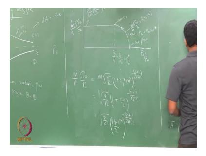
So, if I plot m dot for m dot by a into root T 0 by P 0. So, this is my P b by P 0. So, when P b by P 0 is 1, no flow. When P b is reduced, there you will get a mass flow rate according to this equation, which we have just now derived. So, you would get a mass flow rate according to this equation which would be like this. So, this would be according to this equation which is M dot by A root T 0 by P 0 is a function of Mach number R and T 0.
