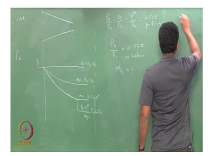
So, what did we do, we had the nozzle here, P 0 equals P b, there is no flow which is also equal to your P exit. If I decrease my backpressure a bit by a small amount, I would get a subsonic flow in the nozzle, which will exit out. So, the exit would be equal to P exit would be same as your P b, but it would be M less than 1 will be mach number at the exit is less than one.
