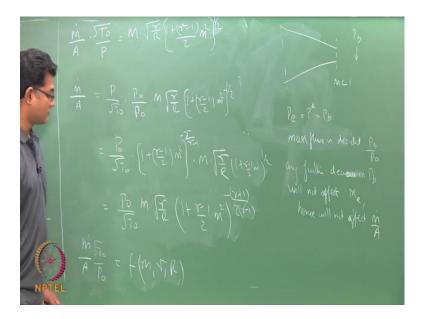
So, my M dot by A into root T 0 by P is nothing but M into root gamma by R into 1 plus gamma minus 1 by 2 into M square to the power 1 by 2. So, this quantity is going to depend only on your mach number at the exit and these things. So, your mach number at the exit is going to depend on these ratios I can change P also in terms of mach number by multiplying and dividing it by P 0, and I write this quantity.
