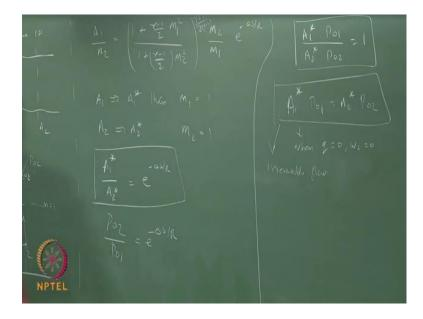
So, we have obtained this particular relation A 1 by A 2, which depends on the Mach numbers of 1, and station 1 and 2, be 1 plus gamma minus 1 by 2 M 1 square divided by 1 plus gamma minus 1 by 2 M 2 square divided by M 2 by M 1. So, this would be gamma plus 1 by 2 gamma minus 1 into e power minus delta S by R. For the process A is A 1 star and A 2 is A 2 star, then my M 1 is 1, M 2 is 1, which tells me A 1 star by A 2 star is e power... So, I have this relation.
