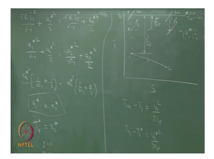
So, I will rewrite that whole thing here, is gamma R T star 1 by gamma minus 1 plus A 1 star by 2 equals gamma R T 2 star by gamma minus 1 plus A 2 star by 2. So, gamma R T 1 is the velocity of sound square. So, I can replace that with this. This would be A 2 star square by gamma minus 1 plus A 2 star square by 2. So, if I take A 1 outside 1 plus gamma minus 1 plus 1 by 2 equals A two star square with the same quantity, it just means A 1 star equals A 2 star.
