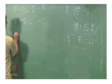
So, d A by A, plus d rho by rho, plus d rho by rho, is m square by 1 minus m square, into d A by A, into v square. So, this is d A by A; there is again 1 by 1 minus m square, into v square; d p by rho; that is the equation for pressure change, which again, I will write it down here. From equation A and B, from equation A and B, I can eliminate my d A.
