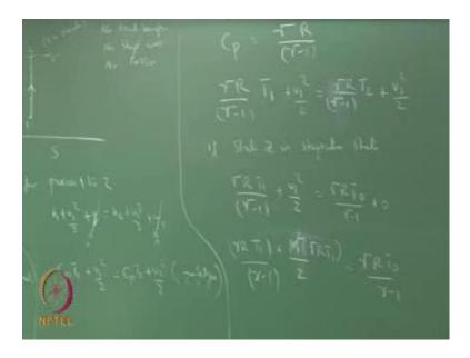
If state 2 is the stagnation state, what do we mean by that I have taken the state 1 to a location where my velocity is now 0. And I have done this assumed these three which means I have taken the fluid from state 1 which has some velocity to allocation where the velocity is 0 isentropically with no heat and no shaft work.
