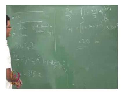
I have a duct at some point here, I have M equals 0.5, T 1 is 300 Kelvin, P 1 is 3 bar, find stagnation pressure and stagnation temperature which essentially means find T 0 1 and P 0 1. So, is the again a mere substitution. We take this relation T 0 1 by T 1 equal 1 plus gamma minus 1 by 2 into M 1 square which is 1 plus 1.4 minus 1 by 2 into 0.5 square, so that would be your T 0 1 which is how much?
