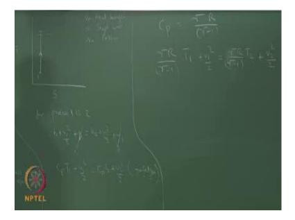
Now let us look at our energy equation. So, in the T S diagram, heat input, heat transfer, no shaft work, no loses. So, in this case between process 1 to 2, my h 1 plus v 1 square
