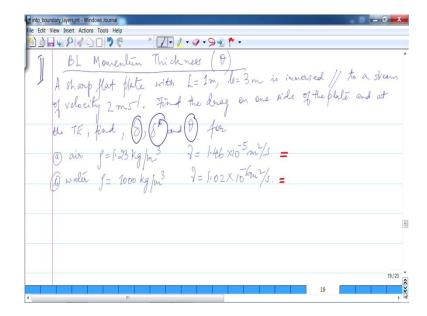
So, this is what we started out doing. So, we said, a sharp plate with length, 1 meter, b, 3 meters is immersed parallel to a stream of velocity 2 meters per second. Find the drag on one side of the plate and the filling edge? Find the boundary layers thickness, which is this boundary layer displacement thickness, which is this and the boundary layer momentum thickness?
