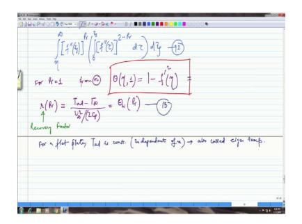
So, this ratio is basically something that I can calculate as a function of this Prandtl number by solving this equation. And this is called the recovery factor and for a flat plate, the adiabatic wall temperature is constant meaning at it is independent of x and hence it is also called Eigan temperature; this where we stopped, OK.
