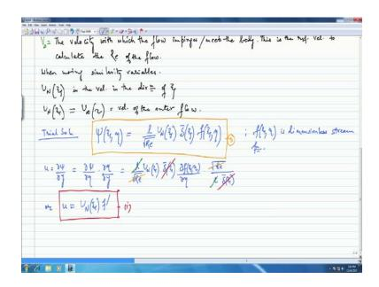
So, V is the velocity, with which the flow impinges or some need, the body. And this is the reference or say this is basically V infinity, I am calling it V infinity. You can basically say a free stream velocity which meets the body and this is the reference
