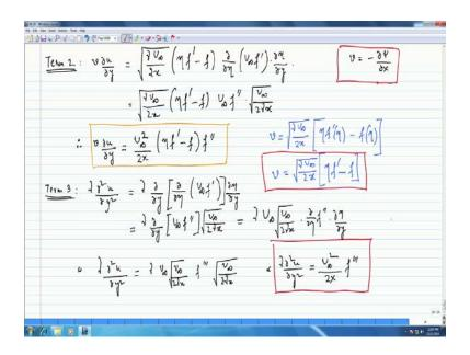
So, what we have here is v; del u; del y, now this is equal to del u del y. So, this is eta; u infinity, 2 x right eta f dash, minus f; del, del eta, u infinity; f dash, del eta, del y. Now, it is important that well; so, I think that you should be able to figure out what I did here, I am not going to elaborate any more. So, u is something that we found out, using the psi like this and so you know what is v? So, v is nothing, but minus del psi del x, so if you
