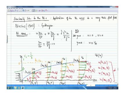
So, where we stopped was; essentially we have the dimensional form of the boundary layer equations, which we are now using.
