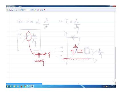
Now, as we kind of, as you must also be aware that shear stress is proportional to the strain rate. In this particular case, in the case of the fluid so d theta by d t is equal to d u by d y. So, therefore, this means that; so, I can write this or shear stress let us denote that by tau is proportional to d u, d y, which is basically the gradient of v horizontal components of the velocity in the wider action, horizontal component in the wider action.
