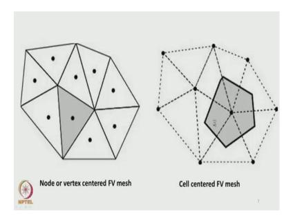
So, we put both these mesh arrangement together, so this is the node or vertex centered finite volume mesh, and this is cell centered finite volume mesh. By now we should able to appreciate the difference between these two type of mesh; so in this, the vertex is centered for the volume and in this cell is centered for the volume.
