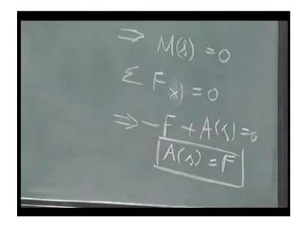
If I take the axial force static equilibrium, I am sorry, I should say F along x is equal to 0, if this direction is x, and this is y. This implies that this is minus F plus a minus F plus a at s equal 0, which means a at s equals f.
