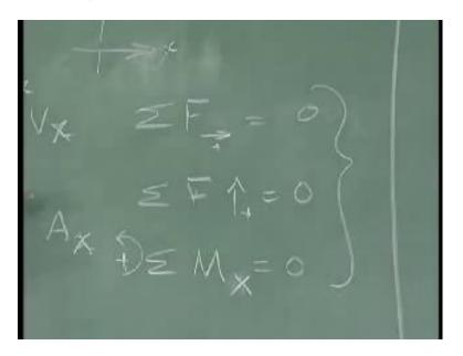
If we are looking at only statics, when we make x equal to zero. Similarly F in the vertical direction is equal to zero and moment; let us take this as positive equal to zero. Three equations can be formed. This can be about any point on this. So, if I take a as the point, or x is the point in question. Then I have three equations three unknowns that I can solve for. So, equilibrium is enough to solve for forces in the member. So, how do we quantify this?
