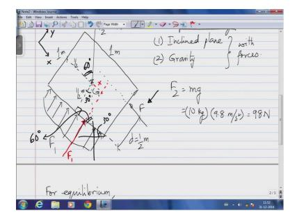
F has a unique line of action, F 2 has a unique line of action, but F 1 is a bit tricky. F 1 does not have a unique line of action which also means that, I need to compute the moment of a distributed force. So, this is kind of distributed force, but what I can do, is I
