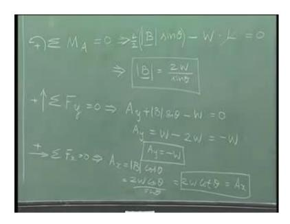
So, I can now write in a very simple way. It is B sine theta minus w. I need to multiply by the length. Let us say this is occurring at half the length of A B C. this is L by two times this minus W times L and this is equal to zero. Immediately, it is possible to solve. I can take out L, B sine theta is equal to two times. So, I will get two W by sin theta. So, now I have solved for the magnitude of B.
