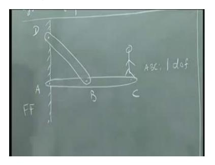
So, this can rotate if I put a hinge over here; which means from three degrees of freedom it becomes one degree of freedom. That this particular platform will have which is just the rotation. And, I wish to arrest the rotation, so that this becomes stationary. The simple thing I can do is to add this particular rigid body, which is pinned at B to the body A BC and pinned at D. So, if I do that this particular body B D has three degrees of freedom.
