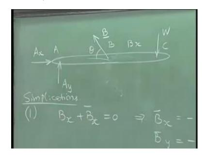
Having done this, one thing that I know here is instead of drawing B x and B y like this, since I have A B vector like this, equal and opposite force can be applied over here. And, what is the direction of this?
