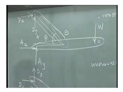
The direction of this is the same as the angle between; the angle between A B and B D; which means, I need to know only the magnitude of this. So, let us now change the unknowns that I have to find out B.
