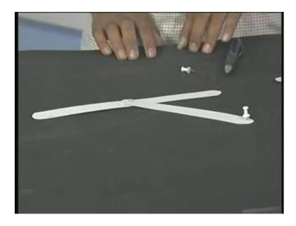
Let us get a physical feel of this particular problem. Let us say this blackboard is the fixed frame of reference. Supposing, I take this particular body A B C and I fix at A to the fixed frame, with respect to the fixed frame the body can only move. I am talking about only planar rigid body. The body can only move by rotating about A. It is very simple. You can have a look at it. And, this is not very difficult for you to make. Just make strips of these sheets and get an understanding.
