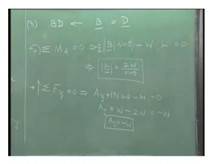
B D we have B equals D. Over the force at B is equal to force at D. Going back to this, can I have any other equation that can be written on this? The answer is no. I have already exhausted all the equations necessary for B D. So, the only thing that is left, the
