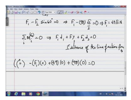
y for this particular instance is 0 because the force F passes through the line of action because the force is half a meter which implies y, which is the distance of the force to the line of actions itself is 0; plus F 2 which is the weight of the body which is 98 Newtons also passes through the center of mass. Therefore, the perpendicular distance to its line of action is also 0. So, for equilibrium we require that F 1 times x with the negative sign plus 49 times 0 plus 98 time 0 equal to 0.
