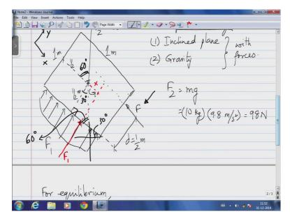
But you know before I can compute the summation of all the forces, F has a unique line of action; F 2 has a unique line of action. But F 1 is a vector key. F 1 does not have a unique line of action, which also means that I need to compute the moment of a distributed force. So, this is kind of a distributed force. But, what I can do is I can replace this with a force that acts at a single point on the bottom of this block as an effective
