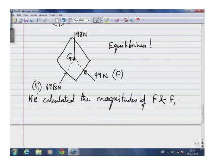
Now, in this process we identified or calculated two forces. Let us differentiate between those two. We identified, we calculated the magnitudes of both F and F 1. So, this is F and this is F 1. Let us understand the difference between F and F 1. What causes F 1? F 1 is a force that is caused by the fact that I have an inclined plane underneath this block.
