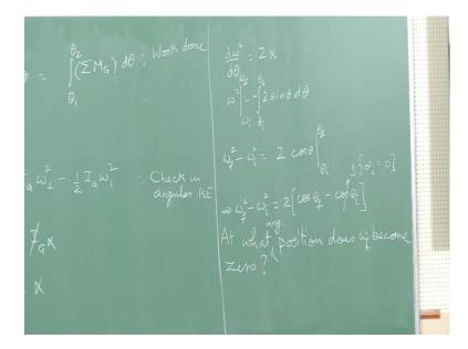
So, d omegas squared d theta equals 2 alpha omega squared is omega squared from some initial omega I to a final omega f. So, now, integrated this is going from some initial theta I to a final theta f minus 2 sin theta d theta. So, this is omega f squared minus omega I squared is equal to the integral of sin theta is minus cos theta. So, that gives this may exists to cos theta and this evaluated in the limits theta I and theta f.
