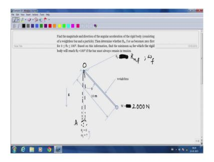
So, let us look at the example here, I have a bar here, it is a weightless bar; that is pivoted at some point O and at the end of the 10 meter along weightless bar, this is a little weight. We will consider this as a point mass for now and this mass is about 2000 Newton's in weight. Initially, it is in a gravitational fields, so if nothing was done to it, it would be at rest kind of in a vertical position like this.
