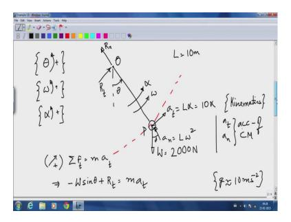
So, let us now draw a free body diagram of this at any other locations. So, this is my O, and this is the body I call this P, this is theta, theta positive, theta this way is positive, this is our sign convention, which also automatically means omega counter clockwise is positive and alpha, angular acceleration counter clockwise is positive. So, let say this is moving with an angular acceleration alpha, this rigid bar O P with the mass at the end.
