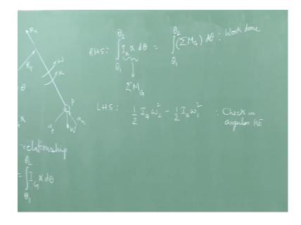
If I am going from some initial state to a final state, then the work done in the angular sense, so this part here, I can replace this part with the sum of all moment about G. So, this part is essentially the work done in an angular sense. This is my right hand side, the left hand side, if I simplifies that, would essentially give me half I G omega 2 squared minus half I G omega 1 squared. And we all recognize that this is the change in the kinetic energy, change in angular kinetic energy.
