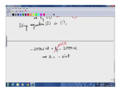
So, minus 2000 sin theta plus R t is 2000 alpha which automatically implies, because R t is 0 as for equation 3, automatically implies alpha equals minus sin theta.
