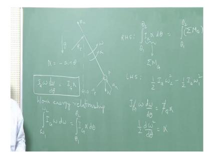
So, we found that alpha equal to minus sin theta. So, that is kind of, that is what we found from the laws of Mechanics. So, now, if I apply work energy concept to this, essentially I omega d omega d theta. So, if I know, if I want to write omega in terms of theta, omega is a function of theta, this is an alternate way of stating our work energy relationship. To bring it into a more familiar form I G W d omega from some omega 1 to omega 2 equals I G alpha d theta from some theta 1 to theta 2.
