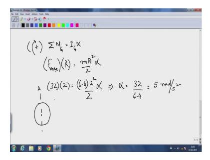
So, let us now also do the moment balance again, I choose to do this about the cylinder center of mass, the only force that causes a moment is the same F max nothing else. So, F max times the radius equals m R square over two times alpha. F max is 32 times the radius where ((Refer Time: 06:58)) is two meters, that means alpha is 5 radians per second square. So, now let us understand what is happening here at this point A, let us understand the kinematic of this cylinder.
