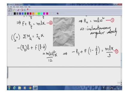
F is a known quantity, I have two equations here, I call this 2, I call this 1 and this is equation 3 I can solve 2 and 3 to find what alpha would be and the corresponding I and the corresponding R sub t.
