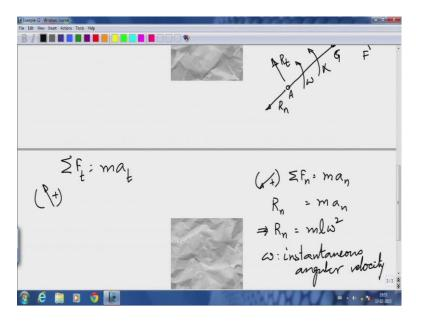
So, what do we learn from this? So, the first thing we will do is apply a force balance. So, if I take all normal reactions towards A to be positive, sum of all normal forces is mass times the normal acceleration. What we find is that R n equals n times a n, which also implies R n equals m l omega squared, where omega is the instantaneous angular velocity. So, now, let us take a tangential force balance, sum of all tangential forces is mass times tangential acceleration.
