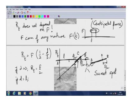
So, what is this mean, if I was a batsman, if I was holding this bat at a particular point and if a ball came and hit the bat at this particular point a distance I over t from the end, I over t from the end. Then, the force I would feel here could not depend on the fact that, there is the force, the reaction force in my hand here does not depend on rather a force up appeared at this point o or not, at this point when the ball hit the rocket or not.
