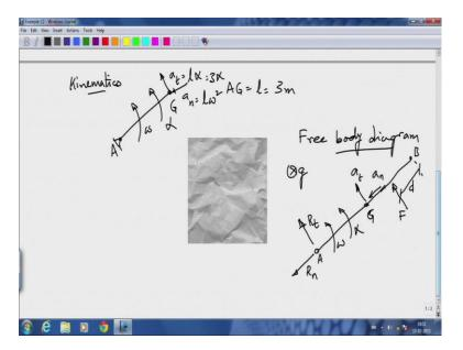
So, let us take that first, the first point that I want to bring to your notice is that, the only part that matters for the kinematics is the distance from A to G. So, if this is rotating at an angular velocity omega and has an angular acceleration alpha and if the length 2 1 is 6 meters, the total length is 6 meters, then this length A G equal to 1 which is 3 meters, which means from the fixed point A, the acceleration of G has two parts.
