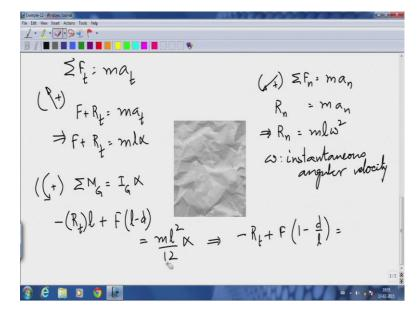
Then, the last equation, we have has to do with the idea, that if I say counter clockwise moments positive, moments about G equals I G times alpha. So, the forces that cause moments ((Refer Time: 07:26)) about G or R t and F, R t causes a moment, F causes a moment, no other force causes a moment about G. So, R t times I causes a clockwise moment. So, in the sense that takes on a negative sign, F on the other hand causes a
