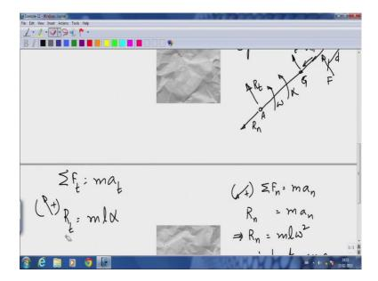
The only tangential force acting on this whole rod with tangential meaning, tangential to the motion are perpendicular to the rod R t equals mass times tangential acceleration, F plus R t equals mass times tangential acceleration. R t is not the only tangential force, there is F as well, so F plus R t equals m l alpha.
