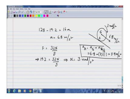
Now, I can solve these three equations, now 128 minus 19.2 equals 16 times a. So, which means a equals 6.8 meters per seconds squared, equation number 3 still valid. So, F equals 32 alpha over 5, which implies 19.2 equals 32 alpha over 5, which implies alpha equals 3 radians per seconds square. So, just to get the feel for how this is going to behave this point here is moving at 6.8 meters per seconds squared and this is rolling at 3 radians per seconds squared.
