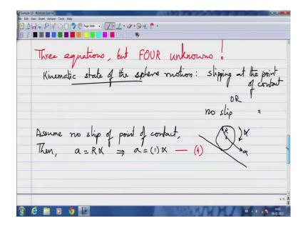
So, this is where we need a little more information on the kinematic state of the sphere motion. So, we going to ask, what is the kinematic state of this sphere motion that is, is it slipping at the point of contact or no slip at the point of contact. So, depending on which of these two is the kinematic state of the sphere motion, our approach from here are on, the 4th equation which we need to complete the system of equations would be different.
