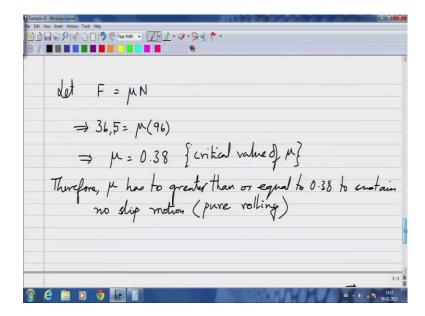
So, if I ask this question, then what I need to do is, relate this F to mu times the normal reaction. So, I shall let F equals mu times the normal reaction. So, 36.5 equals mu times 96, we already calculated the normal reaction N to be mu times 96. So, from here, I can calculate mu to be approximately 0.38, remember mu has no units. So, therefore, we can say mu has to be greater than or equal to 0.38 to sustain no slip motion, which is also referred to us pure rolling.
