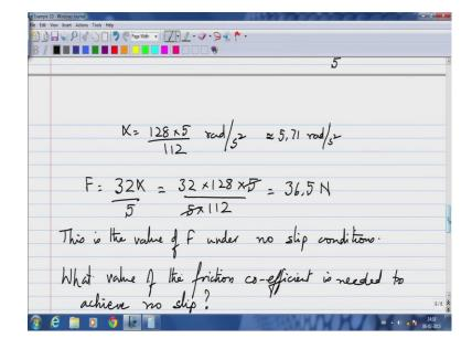
So, from here I can calculate what F should be, F equals 32 alpha over 5. So, this is roughly 36.5 Newton's, so this is the amount of friction needed, this is the friction force acting at the point of contact in order to achieve no slip. So, I leave force inside, this is the minimum value or let me actually say, the way I send it away I complete what I have going to say, this is the value of F under no slip conditions.
