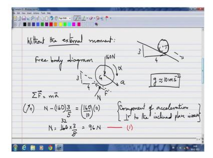
So first, let us look at the case without the external moment, which should be the case of a sphere of sin 1 meter rolling down in an inclined plane. So, let us first draw a free body diagram, I have a sphere, it is the center of mass, this is weight 160 Newton's acting at this through the center of mass. And then at the point of contact, this is normal reaction force, this is the normal reaction force of some unknown magnitude N and a friction force F.
