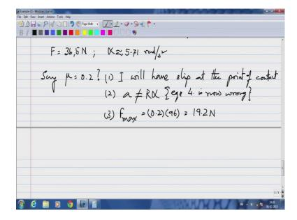
But, what I do now is that f max is now 0.2 times 96, which is only 19.2 Newton's. F max is now 19.2 Newton's, but I need 36.5 Newton's of force at the point of contact to sustain no slip, clearly we do not have. So, essentially these the two surfaces, the sphere and the inclined plane do not have sufficient friction between them, which means we will have slip, which also means that F in the problem, in the free body diagram will take on the maximum value possible.
