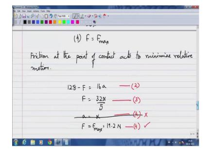
That means the friction force tries to be it is best to minimize relative motion at the point of contact. So, this is the purpose of friction at the point of contact. So, friction at the point of contact acts to minimize relative motion. So, it is going exact it is maximum force, which in this case is 19.2 Newton's and it that force is unable to bring the slip, which is essentially the relative motion at the point of contact 0, it continuous to exert the maximum possible force.
