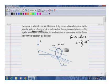
So, let us look at the problem, there is a sphere; that is rolling down in an inclined plane. The inclined plane is 4 on the horizontal and 3 on the vertical, the mass of this sphere is 16 kg or 160 Newton's in force, the radius is 1 meter. There is an external moment that is acting on this sphere in the magnitude of 144 Newton meter. So, I want to first solve this problem without the external moment to see, what we understand and then we will solve the problem with the external moment.
