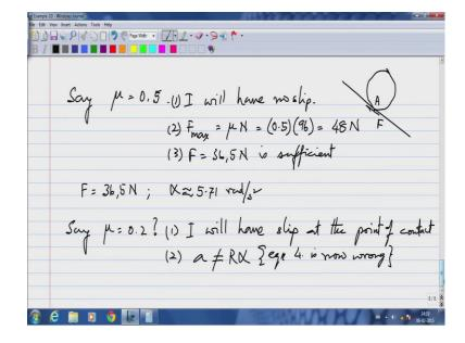
So, let us just do some thought experiments, say mu equals 0.5. So, if mu equals 0.5; that means mu is at least 0.38, mu is greater than the critical value. So, this is like a critical value of mu needed, mu is greater than the critical value. Under these conditions, what it says is that I will have no slip; that is the first observation. The second observation, the maximum value of F as we know from elementary Coulomb friction modeling is mu times N.
