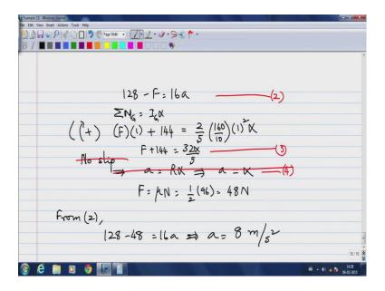
So, what we now have is again I will write down the four equations once more, except this 4th equation is incorrect. Instead what we have is F equals half mu times M, there is equal to half times 96, which is 48 Newton's. So, if F equals 48 Newton's, then from equation 2 128 minus 48 equals 16 times a, which implies a equals 8 meters per seconds squared.
