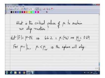
So, I ask the next question, what is the critical value of mu to sustain no slip motion, the answer to that is gotten the equating F equals mu times N; that means, this 666.2 Newton's. I can ignore the sine, because in any case, which are the direction the friction force at the mu calculation would independent of that. So, you can just take the modules of the friction forces equals mu times N, which implies mu would have to be of the value 66.2 divided by 96.
