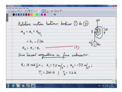
So, we use the laws of relative motion between bodies 1 and 2. So, I will just diagram of this to see, what this spools do together, the body is do together. So, if the angular acceleration of this body is alpha, then at this point A that we said. If the spool rotates an angle theta, then the center of mass comes down a distance 0.5 times theta, which also means a 1 is 0.5 alpha, we have already done that.
