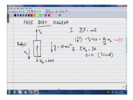
So, let us start drawing our first step is to draw free body diagrams like we said, if there is one skill we walk away from this entire 8 week class, it should be to draw quantitatively accurate free body diagrams. So, just a set of simple assumptions, we assume the cables are mass less. So, they do not have an inertia of their own and secondly, they only sustain intension.
