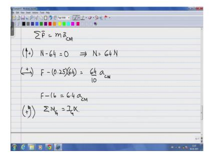
So, let us first do the sum of all forces acting on the body equals mass times the acceleration of the center of mass taking upper forces positive, we are going to invoke equilibrium in the vertical direction which already implies that then magnitude of the normal reaction is not changed 64 Newton's taking horizontal positive, horizontal forces
