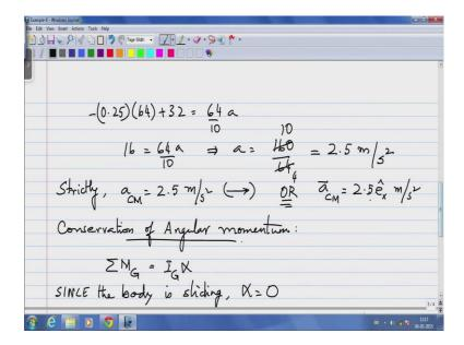
So, minus 0.25 which is mu times 64 Newton's plus 32 equals 64 by 10 times a, so completing this calculation 16 equals 64 a over 10 which implies a is 160 divided by 64. So, this is the acceleration, now strictly the center of mass is what we found to be accelerating at 2.5 meters per second squared. Let us be very clear about that, the law of conservation of linear momentum only determines the center of mass acceleration.
