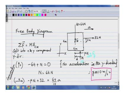
So, we are going do this repeatedly over and over again, if there is one skill you pick up from this entire course at the end, it should be to be able to draw quantitatively accurate free body diagrams. So, this is 4 meters on the side, 4 meters on the side, this is force of 32 Newton's which is my force, the center of mass is a distance 2 meters only this side, the weight of the block acts through the center of mass and that happens to be magnitude 64 Newton's.
