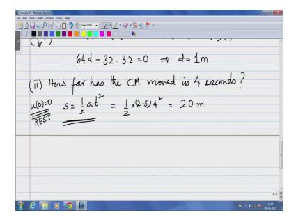
The answer to that is using I Euler's principle of a time integrating for an accelerating body, this assumes that u is 0, u at 0 is 0, this is rest the particle or the block was initially addressed. So, half into 2.5 into 4 square which is 20 meters, so the block has slid 20 meters in the course of 4 seconds of time. Notice, how this equation is what you would usually used for point particle kinematics and we are dealing with rigid bodies.
