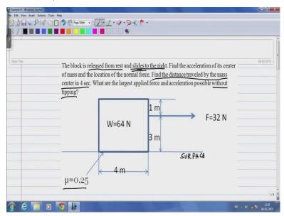
So, let us look at this figure, this is a block of weight 64 Newton's, this is a force of 32 Newton's acting at a distance 1 meter from the top of the block, this block is a square of side 4 meters to 4 meters. The block is on a surface, where the coefficient of section is 0.25, we are asked to find the acceleration the center of mass and the location of the normal force for this condition. So, let us do this, the first step towards solving this problem is drawing a free body diagram.
