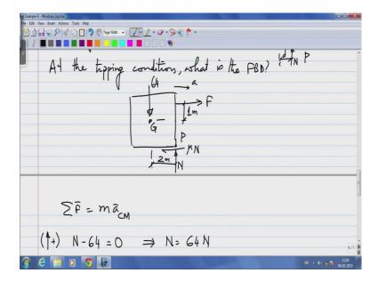
So, let us draw the free body diagram at the tipping condition, the normal reaction whatever be it in magnitude is acting through this point p. The friction force mu times N is still present, the weight of the block is acting through the center of mass and this force F which is now in unknown is acting 1 meter above the center of mass, these are the forces acting on it.
