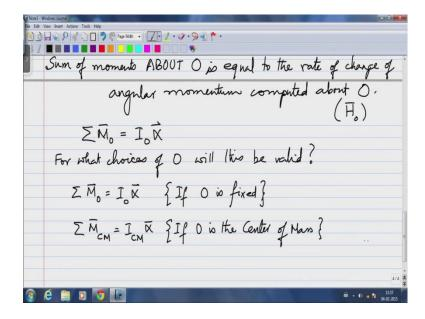
So, we will write it in English, sum of moments about O, so is equal to the rate of change of angular momentum computed about O, an axis through O. So, this second part is what we are referring to as H o and the moment is computed about m. So, unlike angular velocity, moment is a vector, but it is constraint to an axis. So, a moment is calculated about an axis, the axis in this particular instance of plane kinetics is a line passing through O perpendicular to the plane of the paper.
