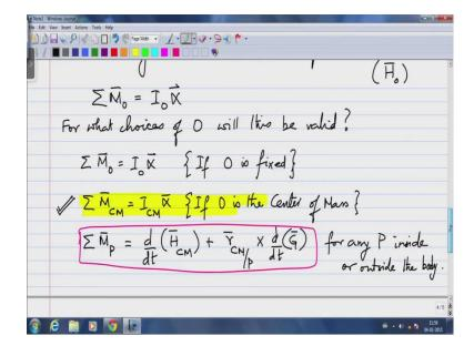
For any other point p, if I have to do this, if I compute the moments about some other point p, then I have to take and additional term involving that distance of this center of mass as observe by p. So, this r bar C M as observe by p is a vector that has a head ending at the center of mass and tail at p and you have to account for an additional cross product, where the rate of change of linear momentum computed of the center of mass is included.
