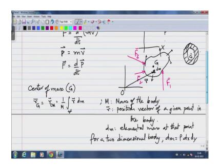
So, the center of mass, we will use the symbol G to denote the center of mass is defined in such a fashion that the integral of r. So, if I take an element d m and r as the position vector of that element d m, so the integral over the whole volume r d m divided by m. This gives me the position vector of the center of mass r the position vector of G. So, here M is the mass of the body, r is the position vector of a given point in the body, d m is the elemental mass at that point.
