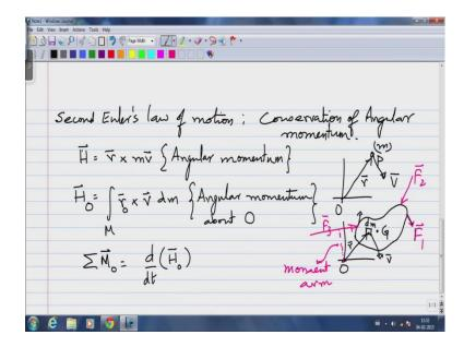
The angular, let say if I have a point particle P again at a point O, this point particle has some linear momentum, linear velocity v and a mass m and if this r is a current position vector, the angular moment is given by r crossed into m v. So, this is what is defined as the angular momentum of the particle, for a rigid body I can define the angular momentum. So, if I have a rigid body and like we said this is center of mass, but different points are moving at the different velocities.
