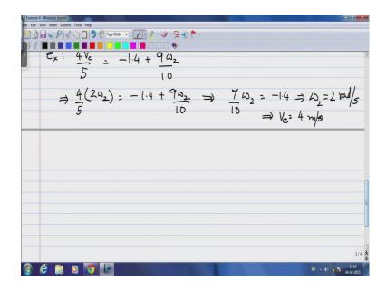
And which also implies V C equals 4 meters per second, so this rod this slider is moving with the speed of 4 meters per second it is of course, constrained to move inside the grove. The rod itself has an angular velocity of 2 radians per second, I will be... I say this once more that the rod has an angular velocity of 2 radian per second, it is not about any point, every point has the same angular velocity about every other point.
