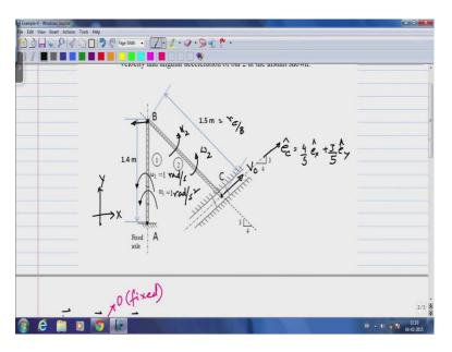
So, here is our first one for today, this is what we will call crank slider mechanism. So, essentially this is a bar A B that is free to rotate about A and there is a pin jointed at D at which the two bars A B and B C meet. Now, C is a slider that is constrained to move on a grove that is on this 4, 3, 5 triangle and we have some lengths. The bar A B, A has a 1 radian per second angular velocity and 1 radian per seconds squared angular acceleration.
