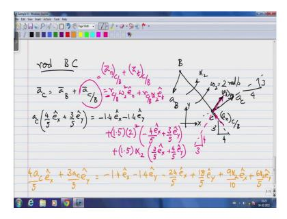
So, now, let us get the acceleration, let us do the analysis for rod B C, again will draw this, the acceleration of B is in some direction C happens to be in that slider. So, the rod B C has, is on the 4, 3, 5 triangle the slider C is constrained to move on a grove that is on a 4, 3, 5 triangle plus 4 plus 3, 5 triangle as shown in this figure. If the slider point C is constrained to remain in the grove it cannot have, because it is only moving on a straight line.
