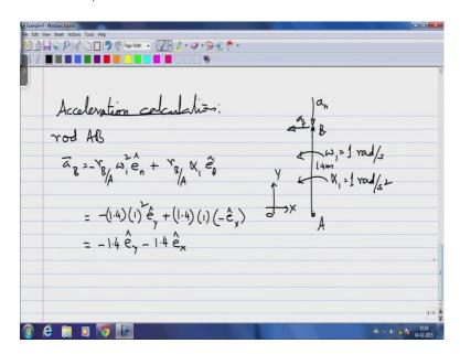
So, now, let us get to the acceleration part, so we will start with the rod A B which translate the information we had in the figure, omega 1 happens to be 1 radian per second and alpha 1 is 1 radian per second squared and this length is 1.4 meters. So, the acceleration of B has two components which is this r of B as observed by A omega 1 square minus e n plus r of B as observed by A alpha 1 e t or e theta. So, just to relay the coordinate system down to get our reference frame.
