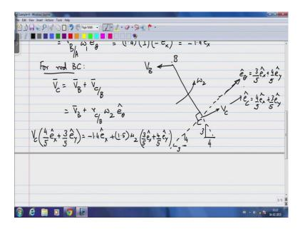
So, this is my bar B C, this is V C it has to be on the unit vector e C equals 4 by 5 e x plus 3 by 5 e y, V B is what we know which is in this direction. Now, if I know that this triangle is on a 4, 3, 5 in this fashion; that means, if I now draw a line perpendicular to that through here, a unit vector along this is my e theta. Because, I know omega 2 is in this direction, so this e theta if this is on a 4, 3, 5 triangle, this would be on a 3, 4, 5 triangle.
