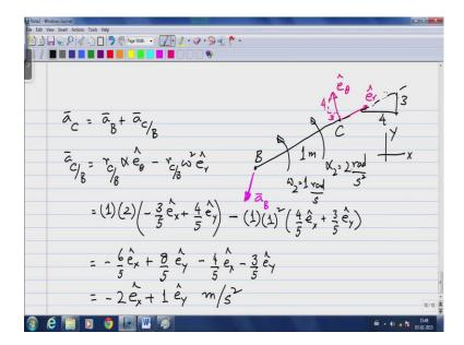
So, let us continue on to bar B C we are told the bar B C is on this 4 through 5 triangle. So, given that e r is along that bar and e theta is perpendicular to it and that as we said will be on a 3, 4, 5 triangle. So, 4 base 3 height is what e r is on 4 height, 3 base is what e theta would be on. We already found the acceleration of B and just for the sway of exactness I am going to draw the acceleration vector exactly the way it came out.
