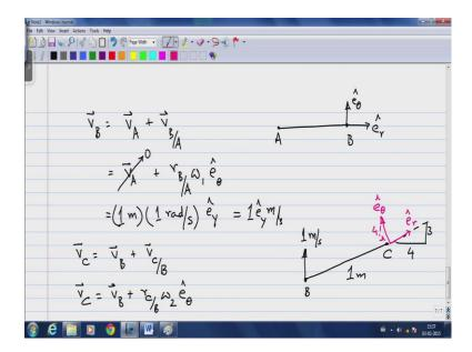
So, velocity of B is velocity of A plus velocity of B as observed by A. So, this is velocity of A which happens to be 0 plus r of B as observed by A times theta dot or omega 1 will use the notation from the figure and that is in a unit vector e theta. So, the velocity of B is simply 1 meter into 1 radian per second and if this is A and this is B, this is e r locally and this is e theta in a Cartesian coordinate system fixed at some point.
