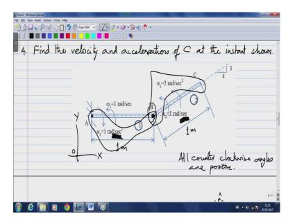
So, this is the fairly simply problem let us move on to a problem involving two rigid bodies that are coupled at some point called B. So, let us look at, let us understand what this is. I have a bar A B where one end of the bar is fixed at A and a bar B C, where the point B happens to be a pin joint that is shade by both the bars A B and B C. And we ask the velocity and acceleration of C at this instant, where the picture is shown.
