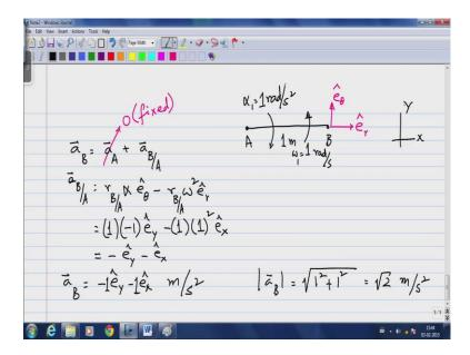
Again I am going to draw this bar A B of length 1 meter, acceleration of B is acceleration of A plus acceleration of B as observed by A. Now, this part has an omega in a counter clockwise sense of 1 radian per second, and then angular acceleration in the clockwise sense of 1 radian per second square. So, this alpha is the same as theta double dot that we had in our previous calculation.
