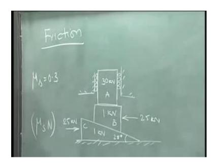
The problem goes like this, there are three blocks A, B, C. The top block is 30 Kilo Newton, I think this is an Engineering problem, where I wish to move this block upward or downward, whatever the case may be. And what they have done is, they have two blocks here with a slanting contact between them. Now, this is the wedge, this is another wedge, but in a block shape.
