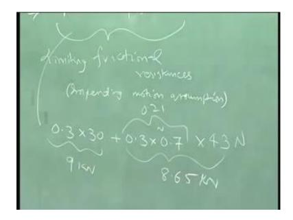
Let just estimate, what could be this, I am go to do a rough estimate here, mu is the 0.3. So, this is 0.3 times 30, this happens to be 9 Kilo Newton and I have a cos theta times mu s that it say plus 0.3 times cross 30. If I take theta to be a roughly 30, cross 30 is root 3 by 2, which is around 0.7, 0.71, 0.7 let us say, this is roughly and this writing. So, this together will give me 0.21 times N, N is given by this with this around 43.
