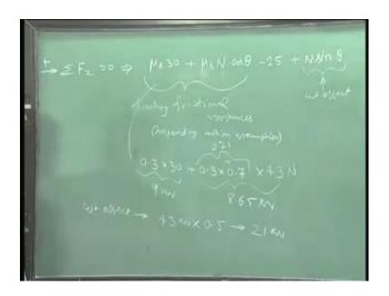
And what is the direction of that; that is also in the positive direction. So, it is plus N times sin theta and this is due to the way that is coming on ward to it. This is due to the weight effect. So, I am separating them, one is the weight effect, the other is frictional effect, of course, I cannot separate the two directly, but just to get an idea, what is the rough value of this, this N is around 43. So, let us this write that also.
