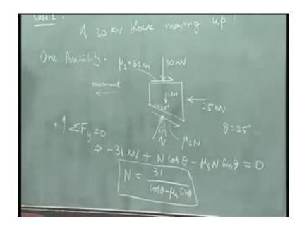
So, let me just draw only the block, I have a slanting contact over here is the 25 Kilo Newton coming inside. Since, there is no side way friction on this block, there is only one vertical force that is acting on the B, block B from A and that is 30 Kilo Newton's. There is no problem and I could have, since it is moving this way, I could have the frictional resistance to that movement.
