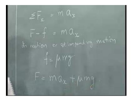
Supposing, it is in dynamic condition then F equals m a, which means that sigma F x should be equal to m times a x. So, if I insert these values, I have capital F minus small f is equal to m times a x, when a x is equal to 0 at this static condition, this is equal to 0, capital F equals small f. But, if a x is non-zero, in the condition when it is non-zero,
