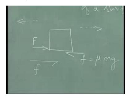
If I have a body like this and I am applying a force F and if I say the impending motion as in this direction, I will apply a force, frictional force. Since, the impending motion is in this direction, it should be opposing it, I will put this f, since it is impending, it is reached the maximum value. I can turn around and say, what if this is negative, I am pushing it a little bit and then, I pulling it.
