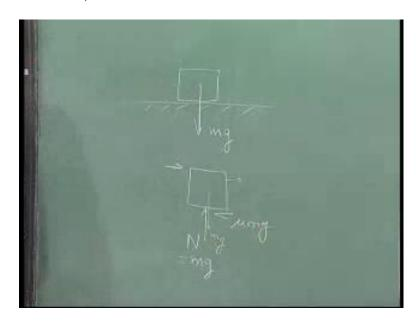
The question is simple, I just have to know, there is a body here, just like what you see here. It has a weight on it equal to m g, I want to know the frictional force on this block, how do you find out. I want to know the frictional force on the block offered by the surface.
