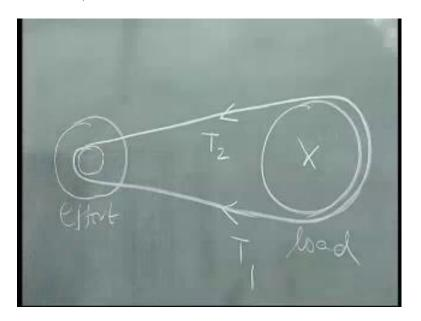
What is a belt drive, let say I have a motor over here, the motor has a roller over here rotor and thus that is rotating, I have another let say this is a wheel, I need to rotate this wheel. So, what do you usually do, I connect is with the belt, let me draw it with another color, I connected with the belt. So, what is basically happening is when this is rotating the friction between the pulley and this.
