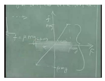
So, if I plot this F versus the frictional force, when I am applying in this direction, let say it is positive, it will keep on increasing this is f, till it reaches mu times m g. Similarly, if I move in this direction, if the impending motion is in this direction, till the motion occurs will keep on decreasing. Again, when it reaches the particular point mu a m g, this case minus mu m g, it will not be moving.
