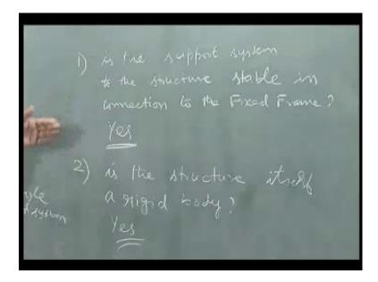
So, the first question that we answer is, is the support system to the structure, here the structure is this which consists of rigid bodies connected together. Is the support system to the structure and stably or stable in connection to the fixed frame? The answer that to the question in this particular problem is yes, if I fix if I inject E and have a roller supported A that is enough to pin this particular rigid body to the fixed frame of reference.
